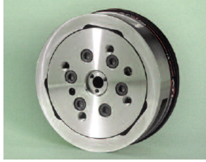
Figure 2.14: ATI Detla SI-165-15 F/T multiaxis sensor used in BLEEX to connect exoskeleton spine to the vest enclosing the user [16, 72]. Diameter: 94.5 mm; Height: 33.3 mm; Weight: 0.913 kg; Sensing ranges: \Xi_x, \Xi_y \pm 165 N, \Xi_z \pm 495 N, \nu_x, \nu_y, \nu_z \pm 15 N·m.
