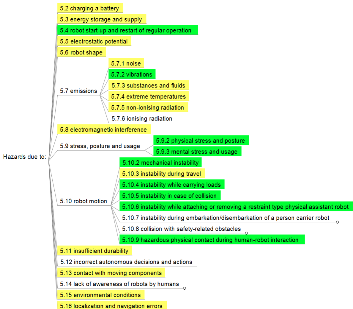
Figure C.1: Sources of hazards in personal care robots (adopted from [68], sections numbers included): green – hazards in restraint-type physical assistant robots relating to the control system, yellow – other hazard sources in restraint-type physical assistant robots.
