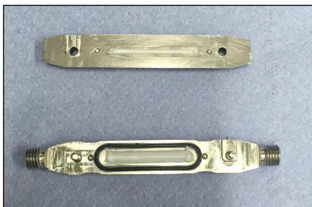
**Figure 27:** A photograph showing both sides of an Anton Paar paste cell filled with sample before being placed inside a vacuum desiccator.
