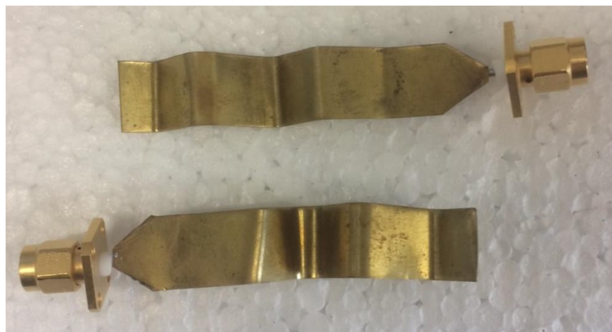
Figure 2.5: A photograph of the monopole antennas used in the small reverberation chamber
