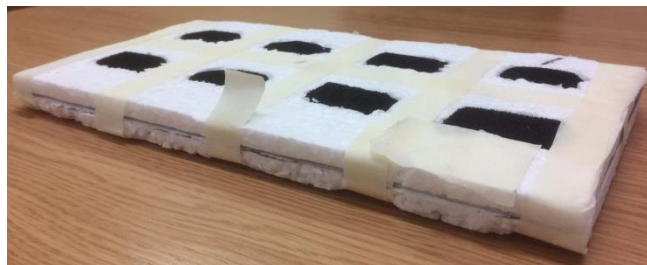
Photograph showing the two layers of polystyrene with the aluminium sheet sandwiched between
