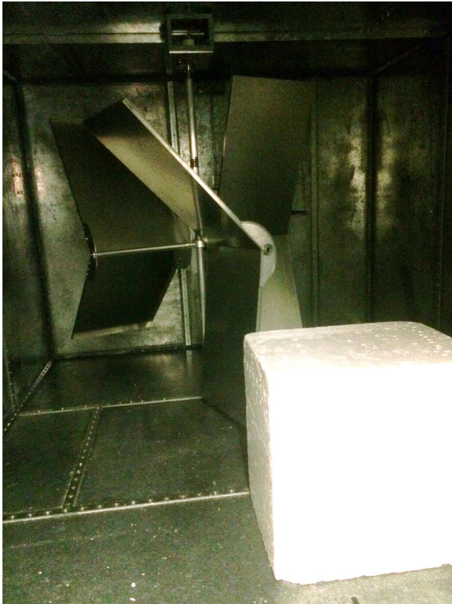
Figure 2.1: Photograph of the Applied Electromagnetics Group reverberation chamber at the University of York. The mechanical stirrer is at the back of the chamber and a polystyrene block is used to place equipment under test in the working volume of the chamber.
