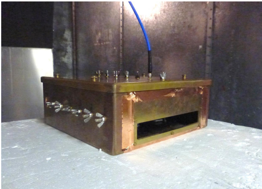
Figure 2.6: Photograph of the enclosure under test inside the large reverberation chamber
