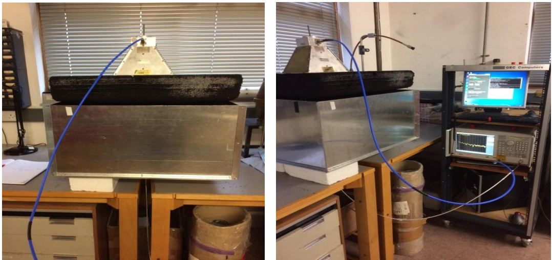
Figure 6.2: Photographs showing the absorber box with the top horn antenna on the left and the absorber box with the coaxial connections to the VNA on the right
