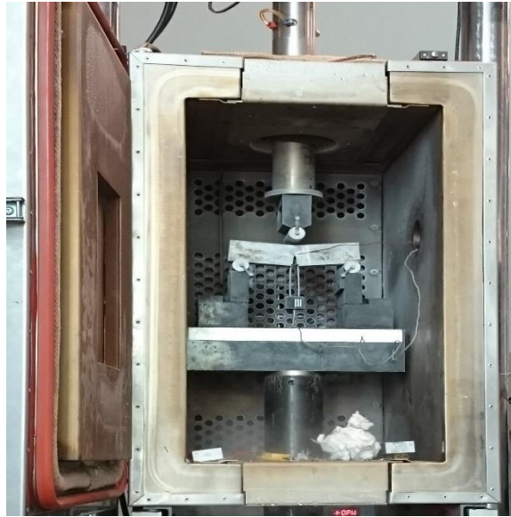
Figure 34 SENB specimen inside the cooling chamber after CTOD testing has been performed.
