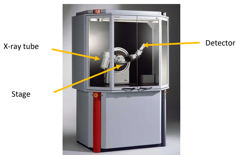
Figure 3-6. Diffractometer Bruker D8 advance used for identification of crystalline phases in CaO-based sorbents [245].
