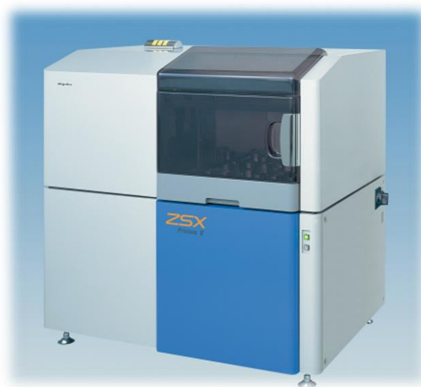
Figure 3-14. Rigaku ZSK Primus I system used for the elucidation of the chemical composition of the CaO-based sorbents by means of the XRF technique.
