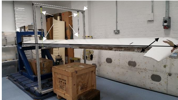
Figure 7.2: The overall wing structure fitted to the metal rig at the wing root
