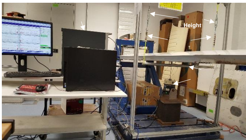
Figure 7.3: Overall experimental set-up with its data acquisition system for the Jabiru wing.
