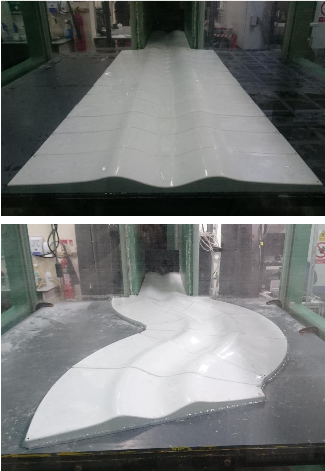
Figure 3.13 Photographs of the straight channel setup (top) and the high sinuosity channel setup (bottom).
