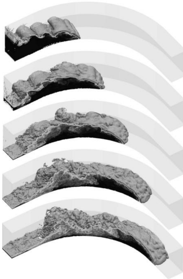
Figure 2.10 The only LES study to date which investigates dynamics in a curved channel [Mahdinia et al., 2012]. A density isosurface visualises the ambient interface as the current traverses the channel. Currently, LES and DNS are too computationally expensive to model complex geometries or larger Reynolds numbers.
