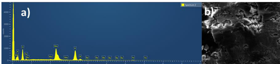
Figure 5.49 Energy dispersive X-ray spectrum of 0.1BF12-0.9K 2 MoO 4 a) is taken from the whole area of b)
