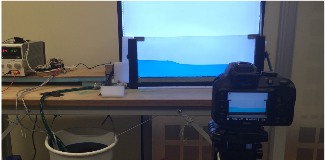
Figure 2.1: Hele-Shaw set up (tank two). Waves propagating in the cell as a result of the operation of the submersible wave-pumps. The Nikon camera was placed in front of the cell and recorded the propagating waves. Two stopping wells (black chambers) are located on the left and the right of the glass plates. A power supply of 12V (white box) is connected to the Arduino.
