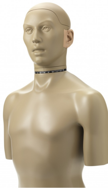
FIGURE 2.15: A KEMAR mannequin developed by G.R.A.S commonly used to generate generic HRTF measurements [69].
