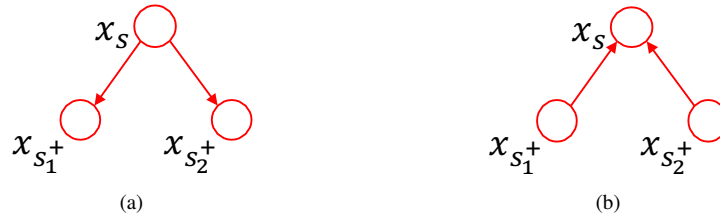
Figure 3.5: Edge directions on cliques in directed tree (a) and polytree graphical models (b).
