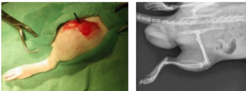
Figure 3.1: Implantation of silver coated Ti-6Al-4V pin in the rat femoral intramedullary canal (left). Confirmation of placement through medial/lateral X-ray (right).
