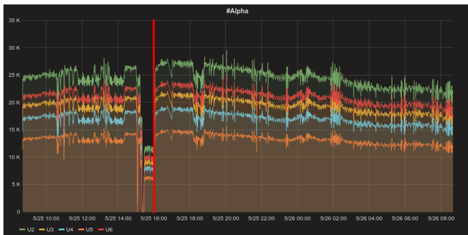
Figure 7.6: Number of \alpha particles observed in five different detectors per 10 s. The full range of the ordinate is 24 hours. A slow downward trend can be observed from the thick red line at 16:00 and forward. This was due to target deterioration.
