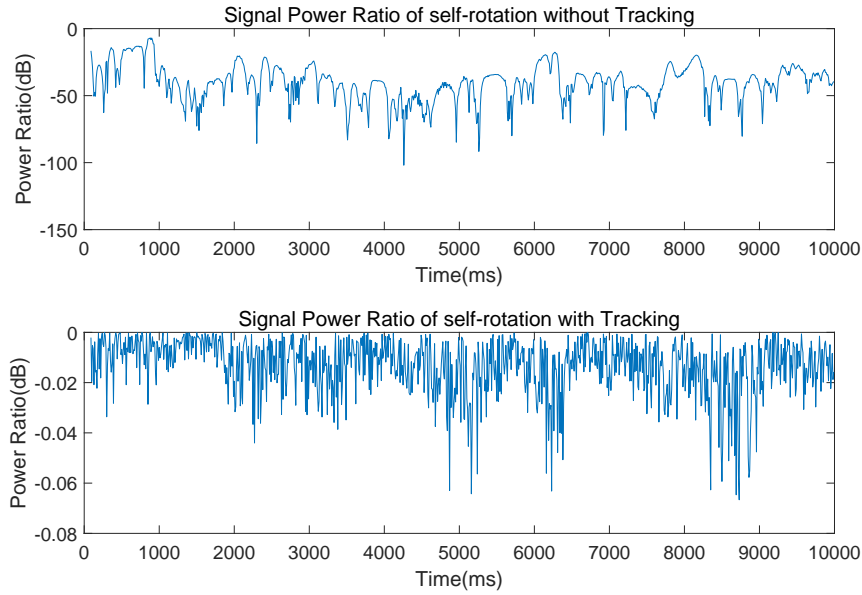
Fig. 3.12: Signal power with and without tracking for scenario 2. The scenario setting is as the same as in Fig. 3.9. Signal power ratio is calculated as the ratio between the received power and the transmitted power.
