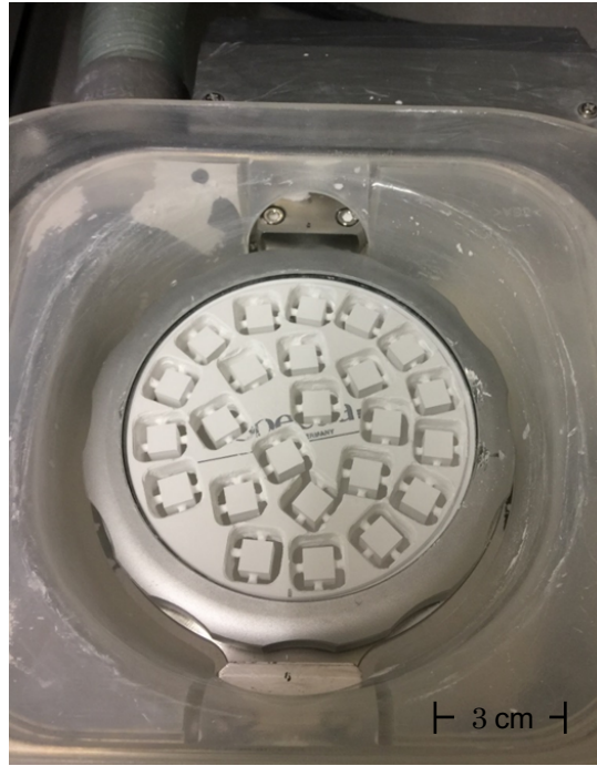
Figure 3: Milling of Y-TZP cubes using DWX-50 CAD/CAM milling machine (Roland DG Corporation, UK).
