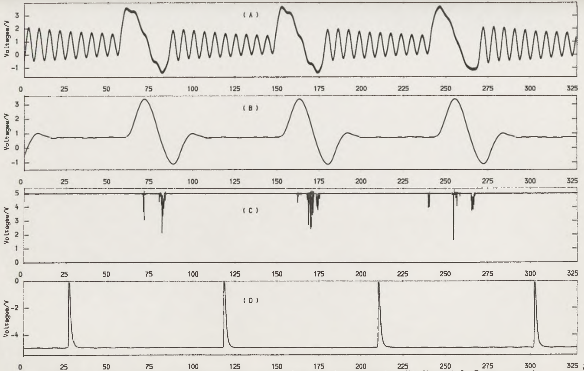
Figure (8.1) The general view of the signals sampled from the four channels. (A) Channel 0: Torque signal, (B) Channel 1: Torque signal after an analogue filter, (C) Channel 2: Voltage across the contact and (D) Channel 3: Cam position trigger impulse (Test speed (650 rpm) at a (105°C) bulk temperature).
