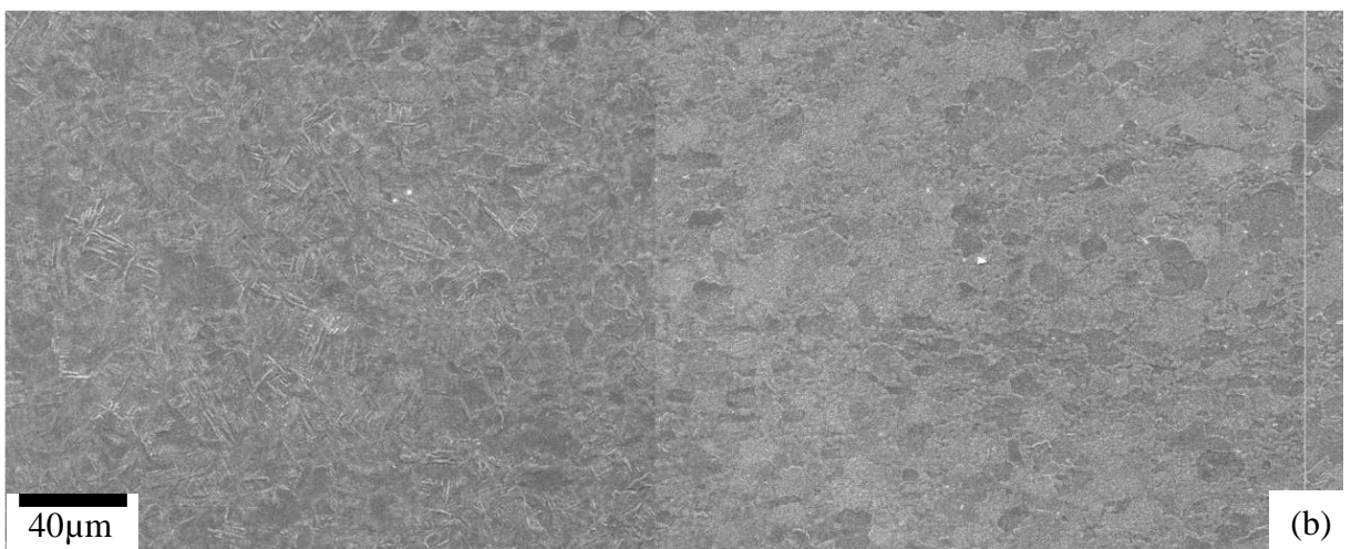
Figure 5.18 Secondary electron micrographs of the bottom transition zone of the weld W20 at (a) the AS and (b) the RS
