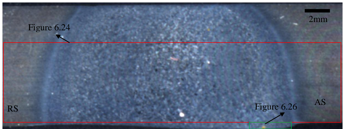
Figure 6.24 Macro section of W19 with red rectangular box indicating the area for EBSD analysis
