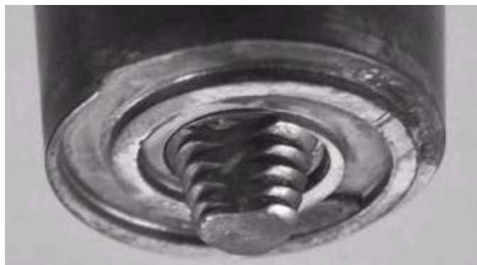
Figure 2.24 Photograph of a scrolled shoulder tool and a truncated cone pin containing three flats (Fuller, 2007)
