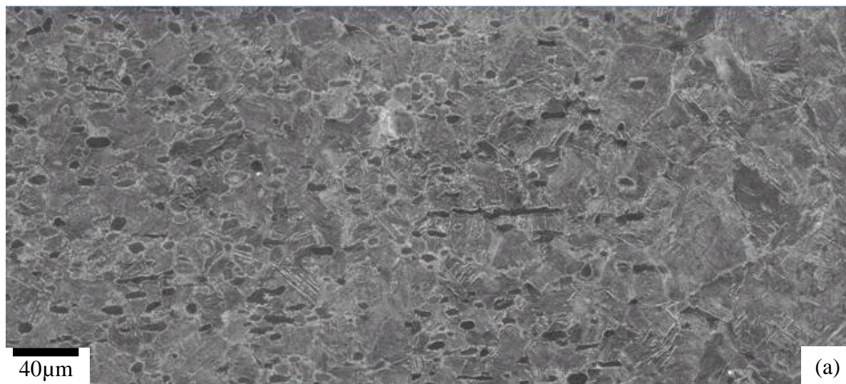
Figure 5.4 Secondary electron micrographs of the surface transition zone of the weld W4 at (a) the AS and (b) the RS
