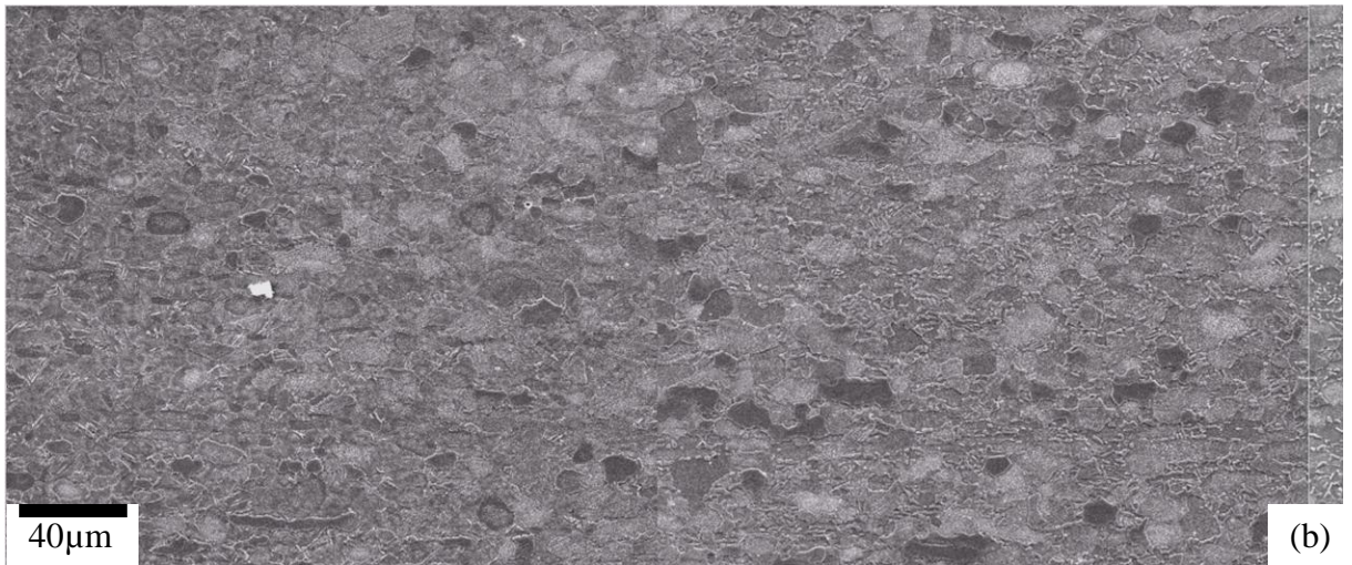
Figure 5.17 Secondary electron micrographs of the centre transition zone of the weld W20 at (a) the AS and (b) the RS
