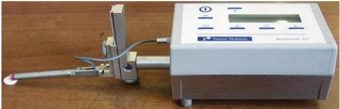
Figure 3.7 Taylor Hobson Surtronic 3+ 9V 112/1590 Surface Tester
