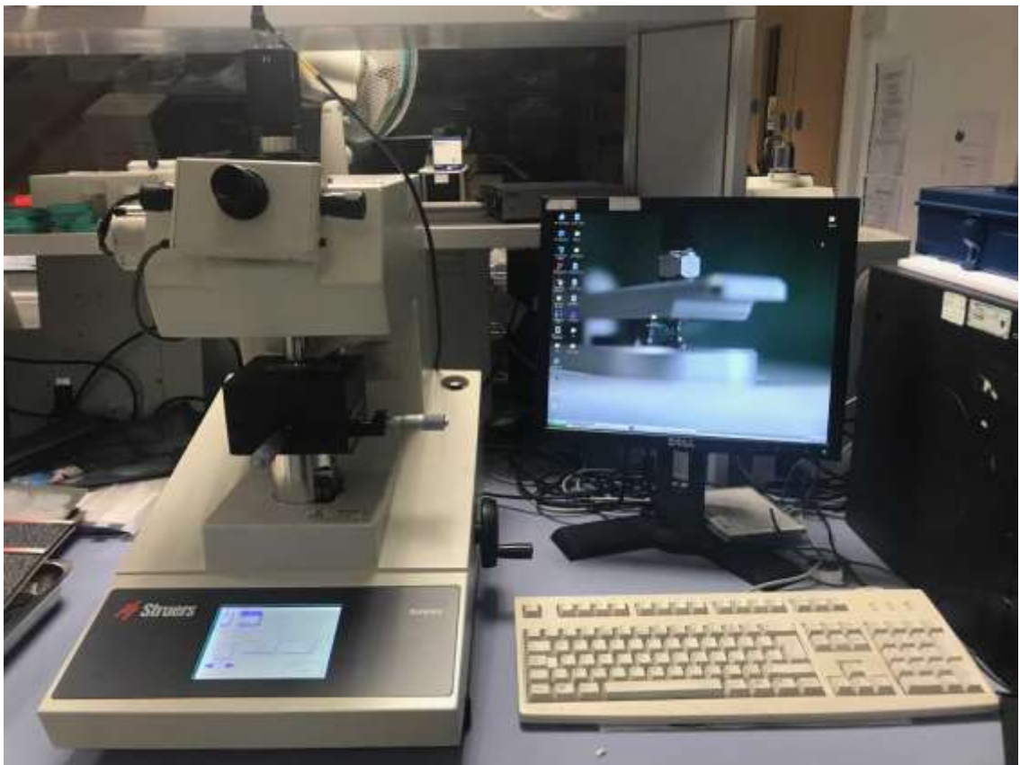
Figure 3-4: The computer-aided Duramin Indenter Machine (Struers A/S, DK 26-10, Denmark).
