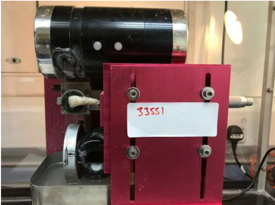
Figure 3-1 Diamond wire saw cutting machine (Well® Walter EBNER, CH-2400 Le Loche).
