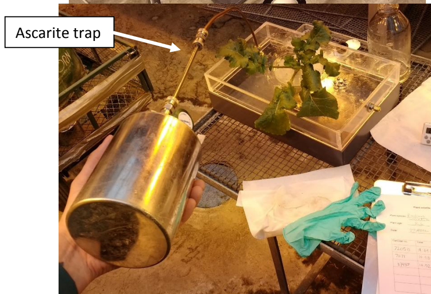
Figure 5.1 Plant volatile sampling chamber. The sampling chamber is depicted in use: A, the assembled sampling chamber set up to sample volatiles from the aboveground biomass of the plant; B, sampling volatiles from the belowground biomass, with the canister and Ascarite trap in place. The hole through which the roots of the plant are separated from the aboveground biomass is covered with a silicon pad and sealed with silicone vacuum grease, to ensure separation of sampling.
