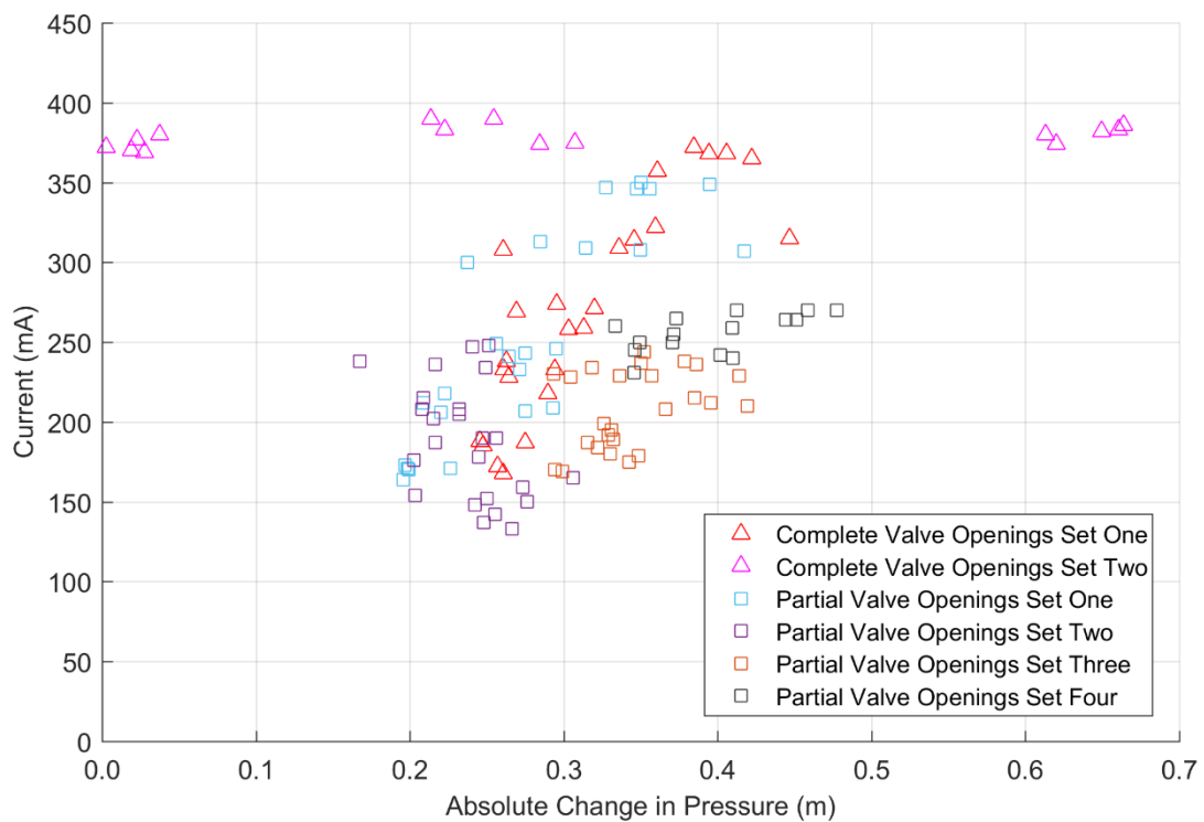
Figure 6.15. Currents at which mobilisation occurred for valve opening transients using ball bearings, against the absolute change in pressure between initial and final conditions.
