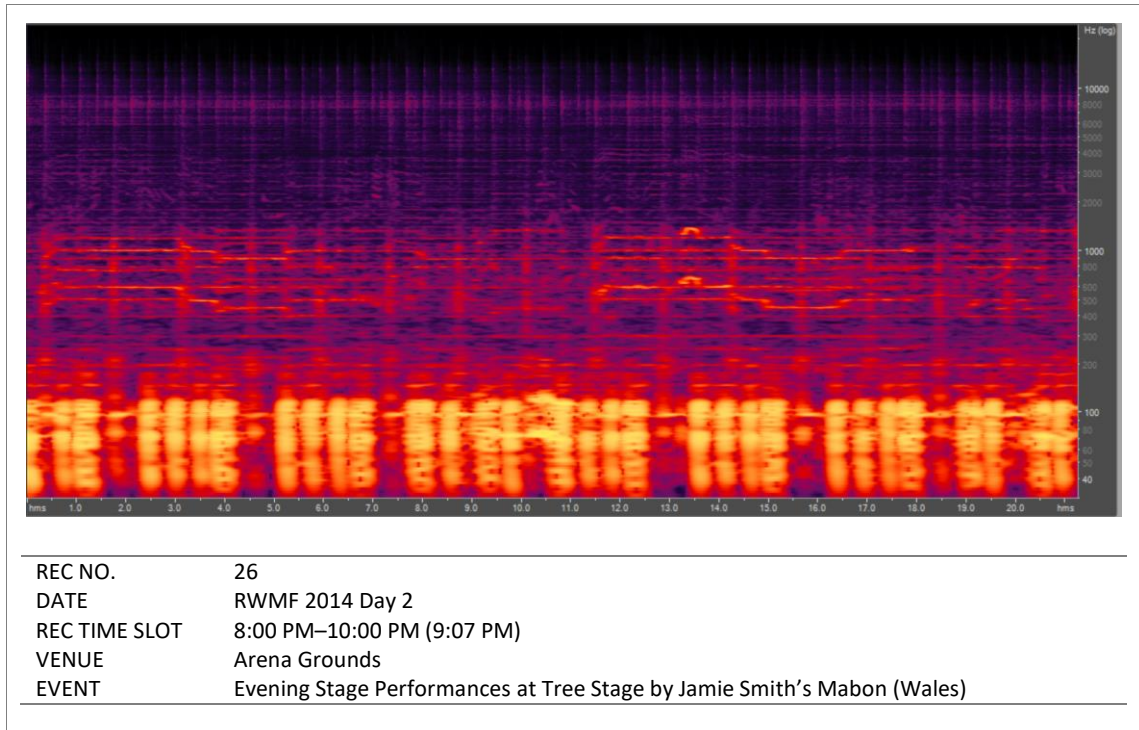
Figure 4.37: Excerpt of frequency spectrogram during the Evening Stage Performances at the Arena Grounds. Low frequencies of music appear at 40–120 Hz. (Full recording: Rec No. 27)
