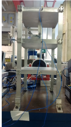
Figure 5.6: Experimental setup for the representative three storey building structure.
