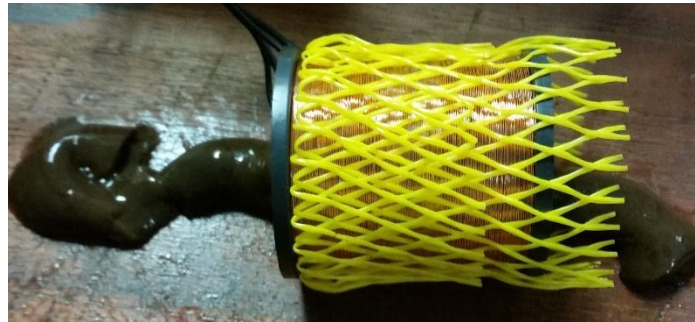
Figure 28: Fluid-like nature of 14 mg/ml ferrogel, which had a tendency to leach out from both sides thinning the diameter as it did.
