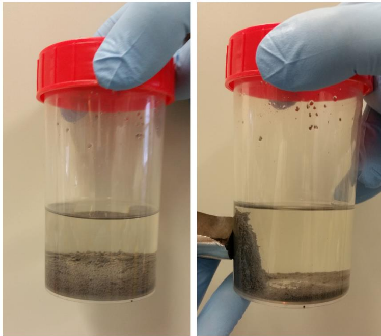
Figure 43: Microcarriers displayed strong attraction when a magnet was placed in close vicinity of them.
