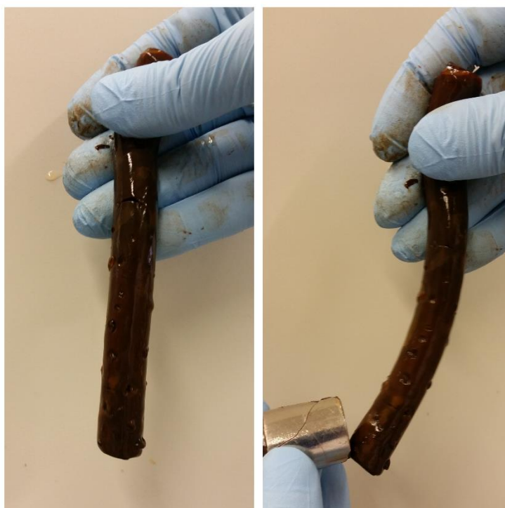
Figure 15: The image demonstrates the ferrogels magnetic properties using a neodymium magnet.
