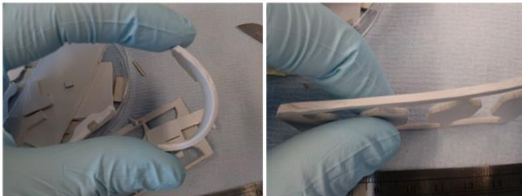
Figure 39: Image of 50:50 EHA:IBOA poly-HIPE with 9 wt% carbonyl Iron particles and 75% water content (Left) and 90% (Right).
