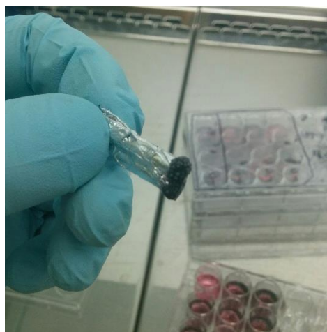
Figure 58: Magnets wrapped in a sterile foil sleeve, which can be easily removed using a sliding motion. Any particles attached drop on to new culture surface.
