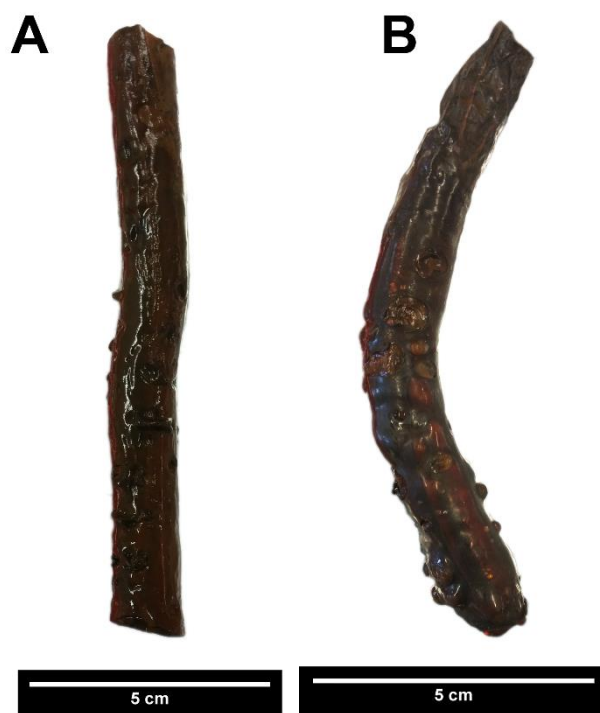
Figure 23: In situ developed ferrogels showing A, the fully hydrated state at room temperature and B, the collapsed state at approximately 45°C.
