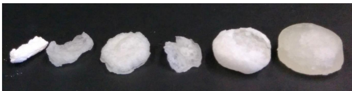
Figure 29: variation of quality during the initial phases of the project. The appearance on the right-hand side shows an oil retaining Poly-HIPE after several attempts of washing. Other parameters such as changing the oil and using a solvent, which was highly miscible in the oil later, improved the quality.
