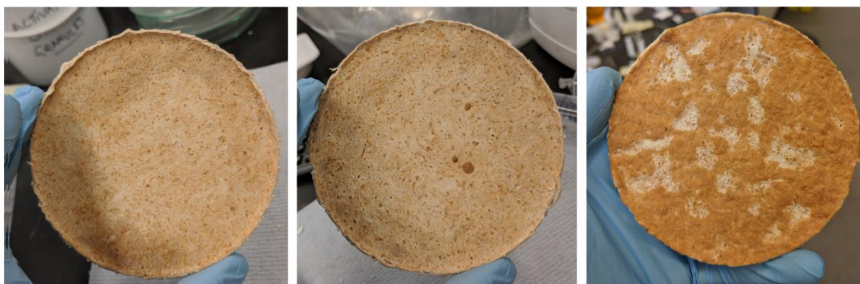
Figure 65: EHA-IBOA poly- high internal phase emulsions with added wood fibres (From left to right): 5 wt% and 70% water,
