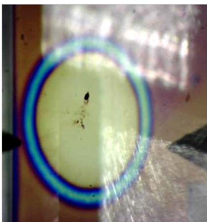
Figure 7. 3: a) An image through a 10 times objective lens of an area of a spray cast PEDOT:PSS film demonstrating the reticulation of the film. b) A dektak line scan from the centre of the reticulated area, in which the PEDOT:PSS has entirely dewetted, across the thick outer ring.
