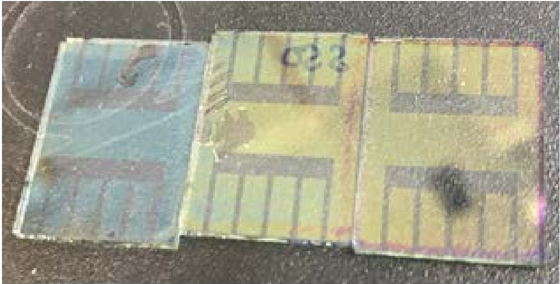
Figure 7. 15: Picture of films of spray cast LEP from 80:20 solvent blend Chloroform to Mesitylene. The films were deposited at a base plate temperature of 25 °C, pass speed 50 mm s -1 , pass height 40 mm, fluid pressure 40 mbar and solution concentration of 4, 5 and 6 mg ml -1 from left to right. The central film was scratched in order to measure the thickness.
