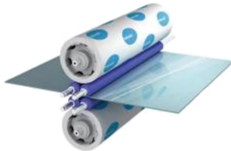
Figure 2.1: An example of the cleaning process developed by Teknek. The pale blue surface is the surface to be cleaned (it is grey in the left part and bright in the right part after the removal of the particles); the four blue rollers in contact with the surface are the cleaning rollers and the two big white and blue rollers are the adhesive rollers. Image courtesy of Teknek.
