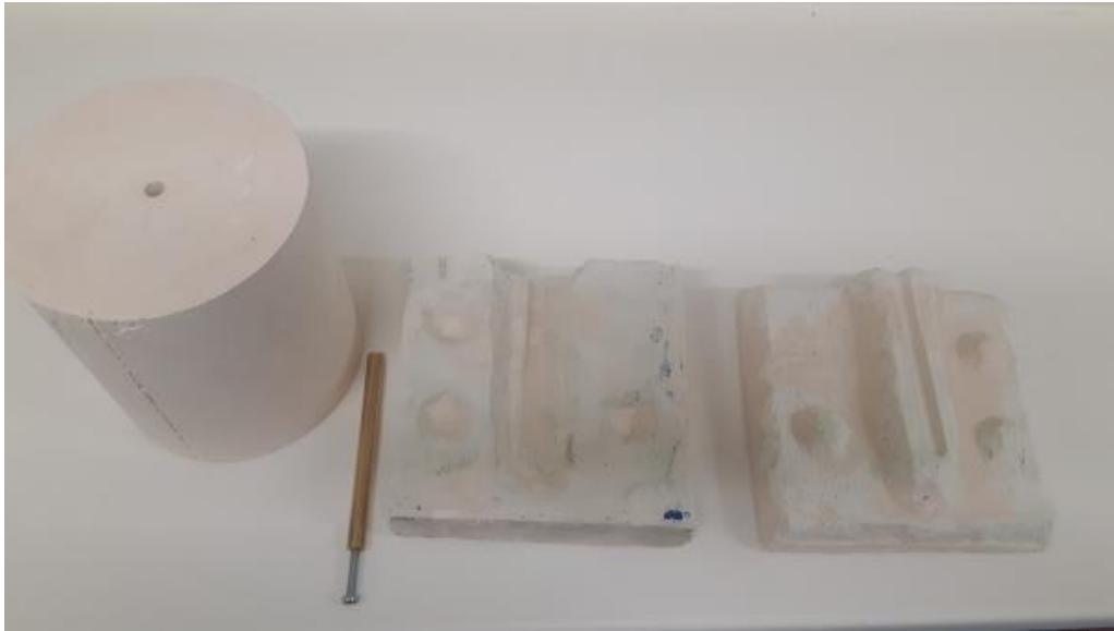
Fig. 6.1.1 – New moulds and the former made to be more dimensionally correct for fuel rods.
