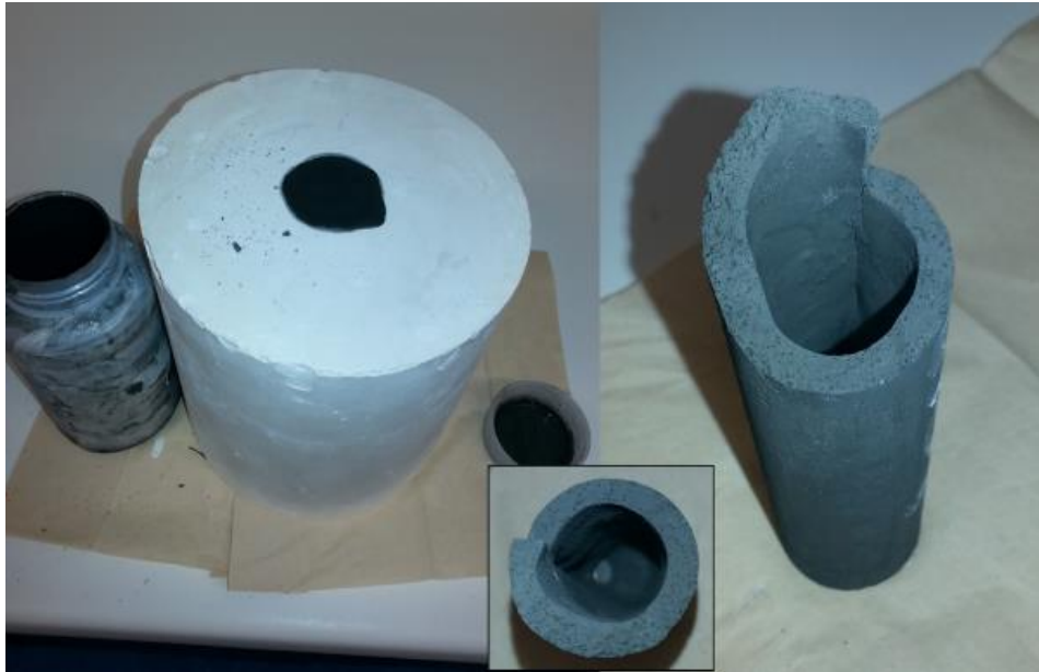
Fig. 6.1.2 – Photographs showing the initial mould used (left), with the largest intact piece shown from the side (right) and the top (middle inset).
