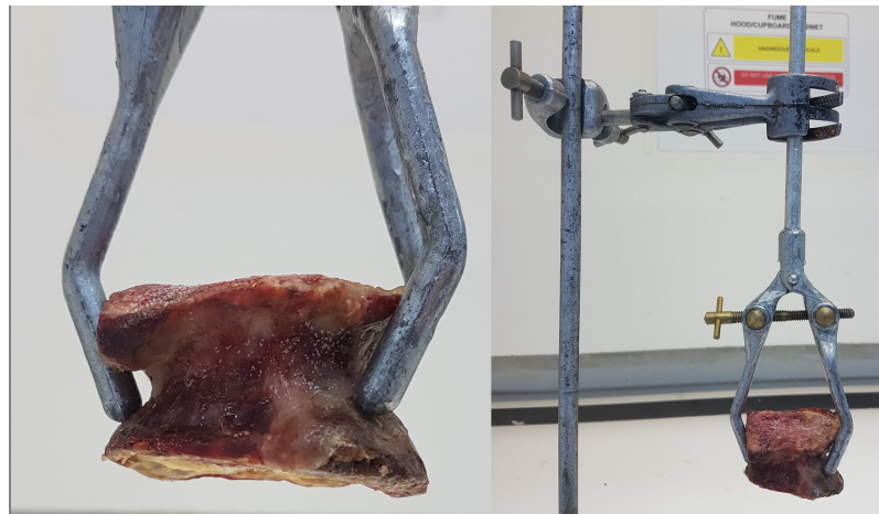
Figure 3.2: The holding of the vertebrae during potting in PMMA endcaps.
