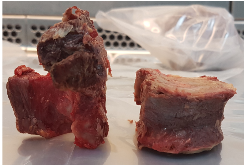
Figure 3.1: The removal of the posterior elements, through cutting at the narrowest part of the pedicle.
