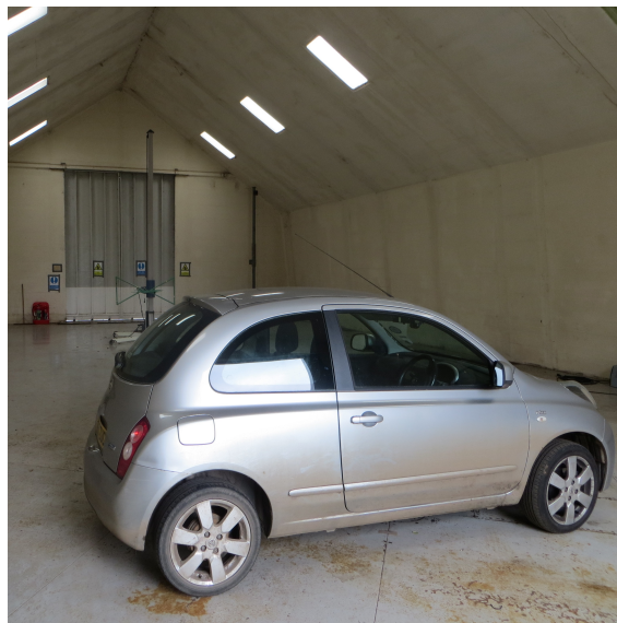
FIGURE 2.3: CISPR12 OATS Typical Arrangement. Located at HORIBA MIRA, Nuneaton.
