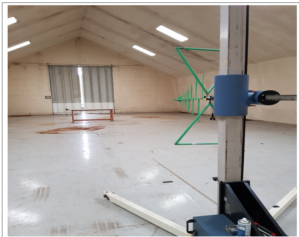
FIGURE 4.21: Electrically Large Source, Wire Harness, Height Scan Measurement Setup
