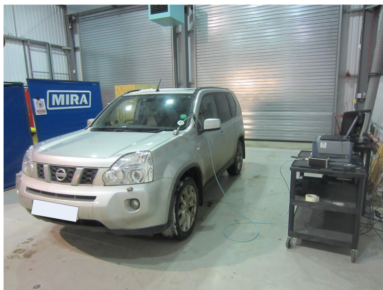
FIGURE 7.23: Surface Current Probe Measurement Equipment Setup
