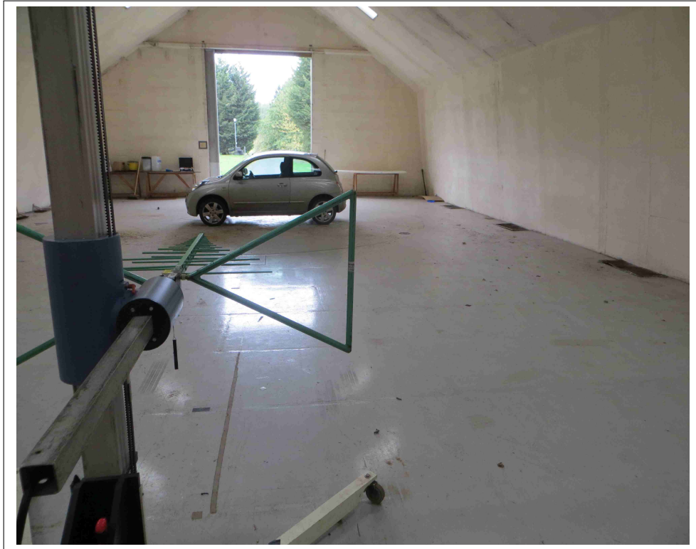
FIGURE 4.20: Electrically Large Source (Nissan Micra), Height Scan Measurement Setup
