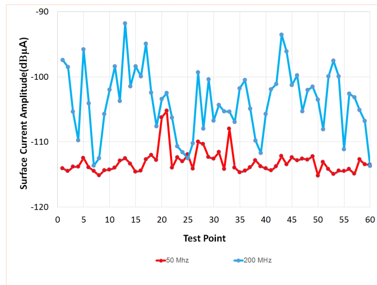
FIGURE 7.24: Surface Current Amplitude Recorded at 50 MHz Compared of to Amplitude Recorded at 200 MHz
