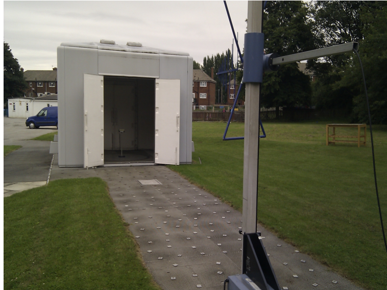
FIGURE 2.2: CISPR12 OATS Typical Arrangement. Located at Eurofins Castleford.
