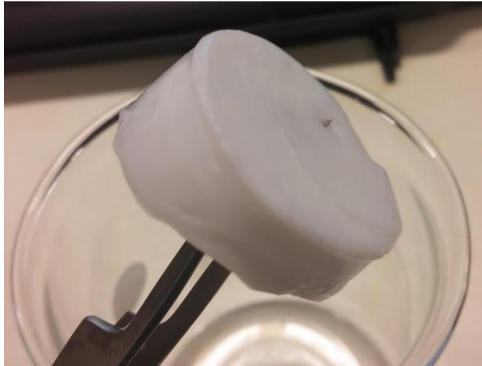
Figure 3.1: A crystallised 10%wt aqueous solution of sodium myristate.
