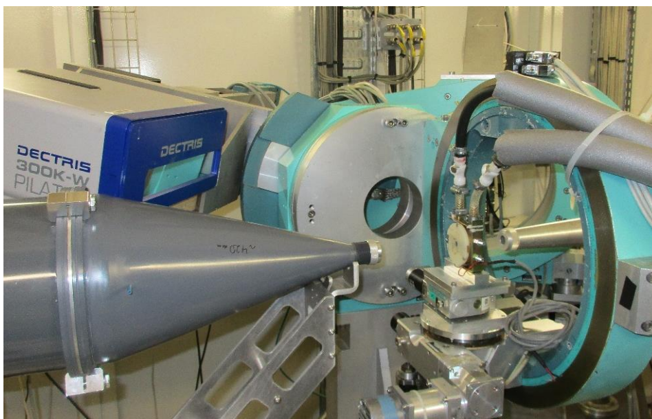
Figure 5.3: The capillary stage used at BM28 at ESRF
