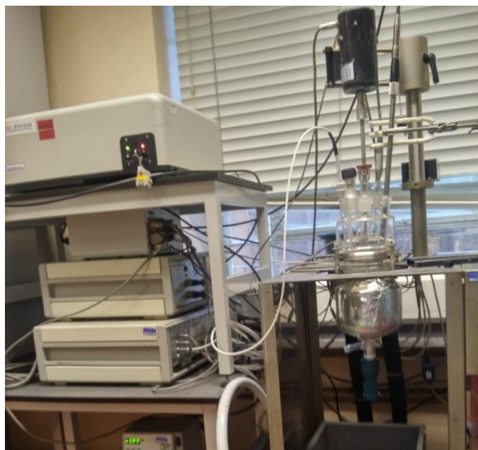
Figure 5.1: Simular 0.5 L reactor from HEL Ltd with RamanRXN1 system from Kaiser Optical systems used for in-situ measurements
