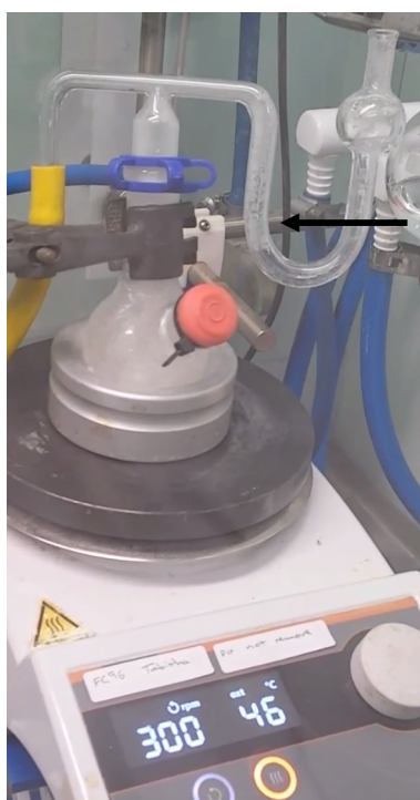
Figure 3.22: The moment of eruption during the Baeyer-Villiger oxidation using H 2 O 2 (30%) and water only. H 2 O 2 (aq) was initially added at 0 °C and then heated. When the mantle temperature reached 46 °C, a sudden and violent expansion occurred. Arrow: the cloudy reaction mixture can be seen making its way through the bubbler tubing.
