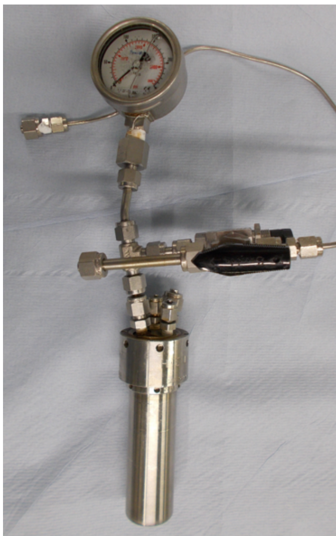
Figure 3.30: Larger size autoclave used for scale-up hydrogenation with a maximum safe pressure of 200 bar.
