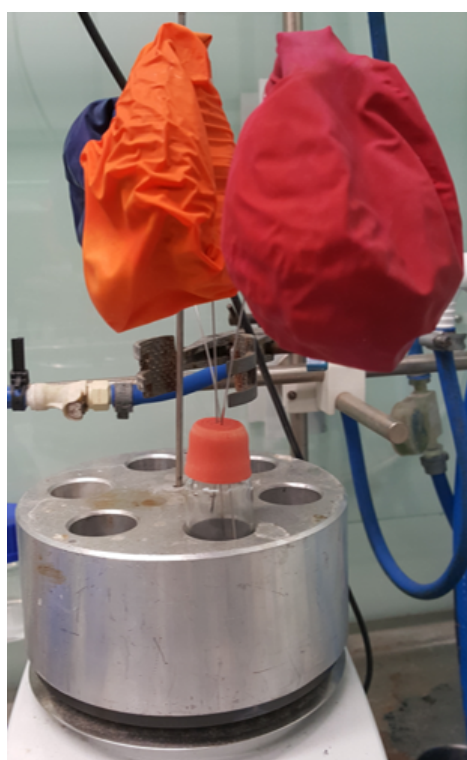
Figure 3.31: A simple set up for the hydrogenation of lactone 1b .
