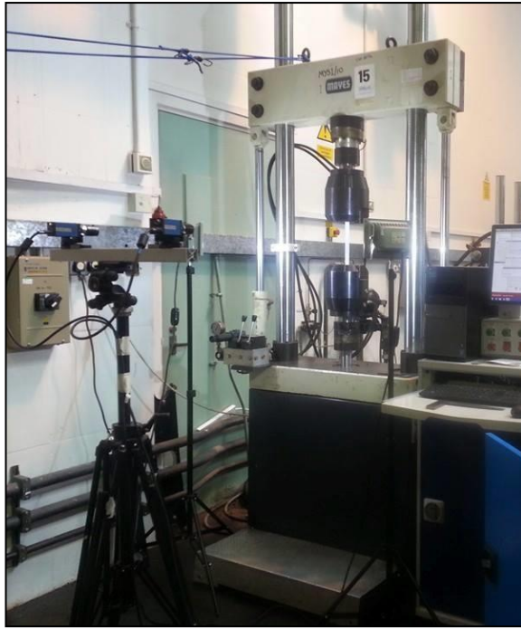
Figure 3-7 3D DIC set up for standard tensile test (left) and 3D DIC set up for a forming/punch test (right).
