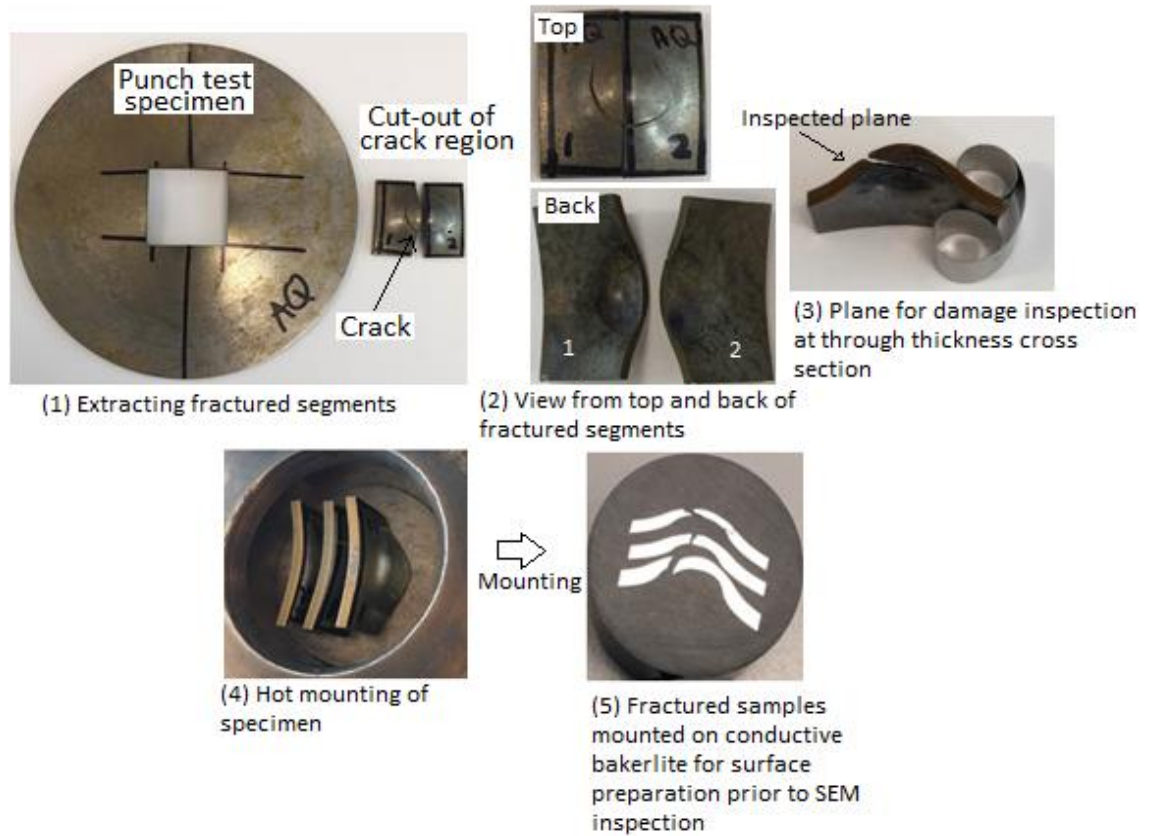
Figure -5-14 Centre region of a failed punch test specimen is extracted out and later is cut in half to reveal the cross-section profile of a failed punch test specimen.
