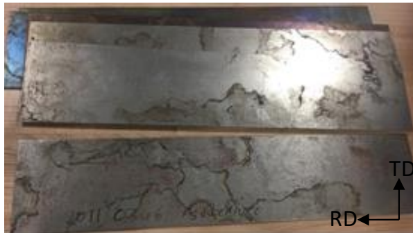
Figure 3-1 DP1000 sheet steels which are being used as research material in this study. Samples for every tempering conditions samples are received in sets of four with an approximate size of 120mm x 550mm x 1.6mm (width x length x thickness).
