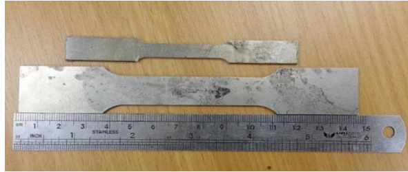
Figure 3-8 Example of two tensile specimen geometries after being cut using the EDM. At the bottom is the 12.5mm width standard specimen and the top (smaller) one is the 6mm wide subsize specimen.
