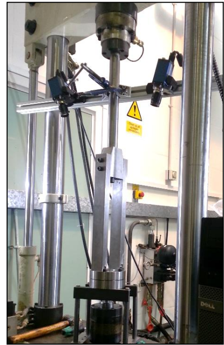
Figure 3-7 3D DIC set up for standard tensile test (left) and 3D DIC set up for a forming/punch test (right).
