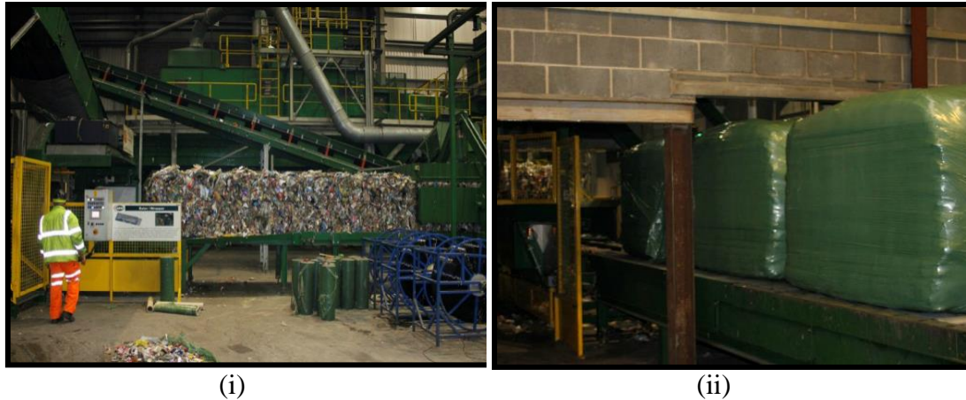
(i) (ii) Plate 3. 5: The waste facility showing (i) RDF conveyed to the bale wrapper and (ii) RDF bales for export (AWM, 2011).
