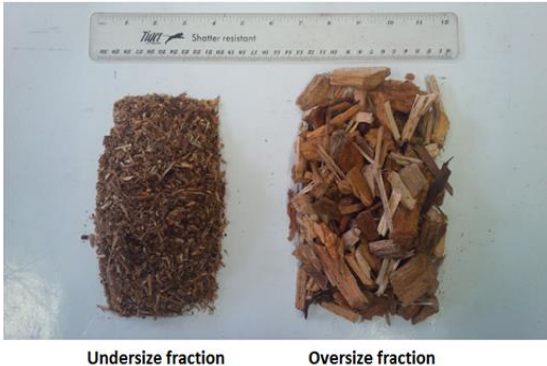
Plate 3. 9: Undersize and oversize fractions of woodchips obtained with the 4.75 mm mesh size sieve.
