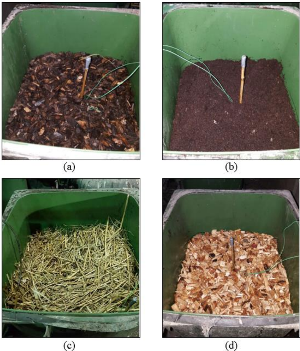
Plate 8. 1: Media materials used in the biofilters on site: (a) old woodchips in BF1, (b) peat in BF2, (c) wheat straw in BF3, and (d) new woodchips in BF4.
