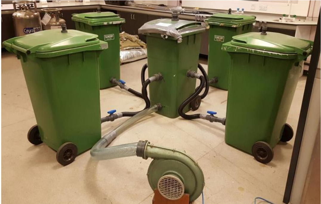
Plate 3. 6: Fabricated pilot-scale biofilter system in the laboratory.
