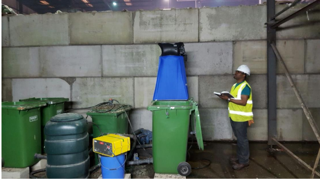
Plate 3. 7: Airflow rate measurement using an Alnor Balometer (blue cone) through the pilot-scale biofilter.
