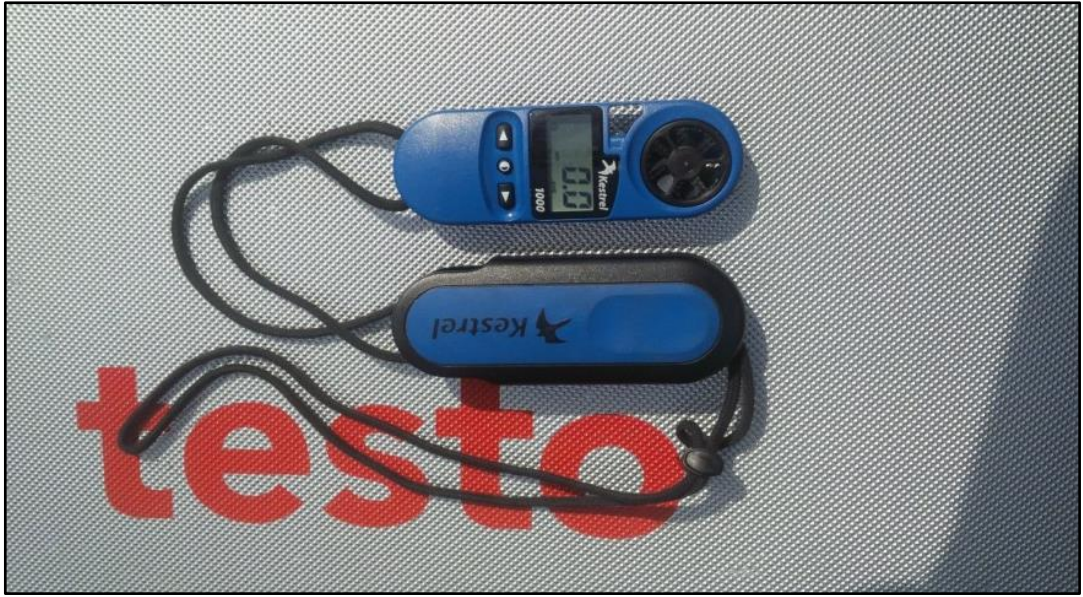
Plate 3. 22: The Kestrel ® 1000 Pocket Wind™ meter.
