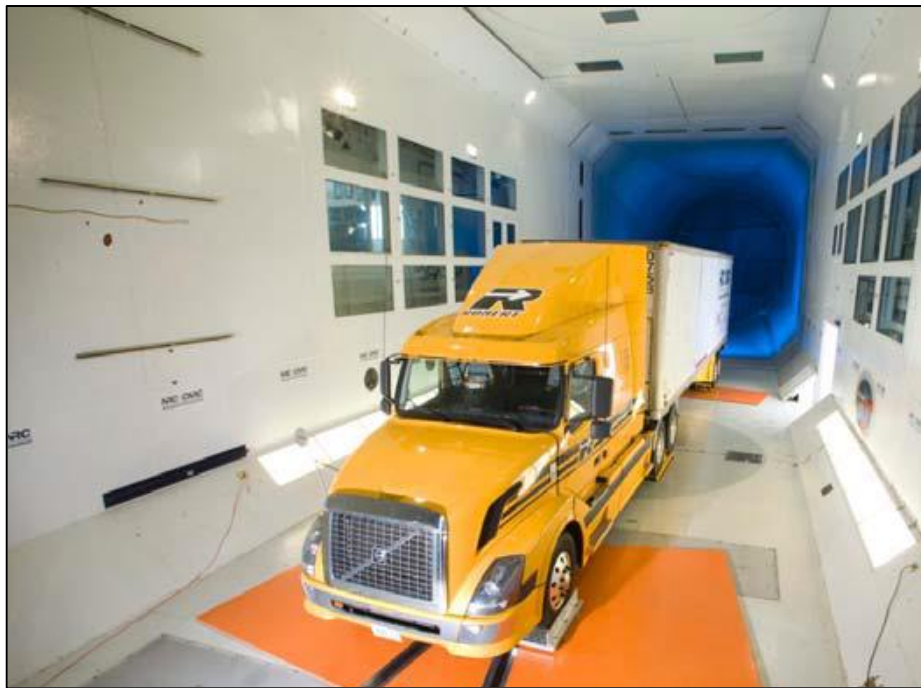
Figure 2.32: Class-8 tractor-trailer in the National Research Council of Canada. Full-scale wind tunnel [51]
