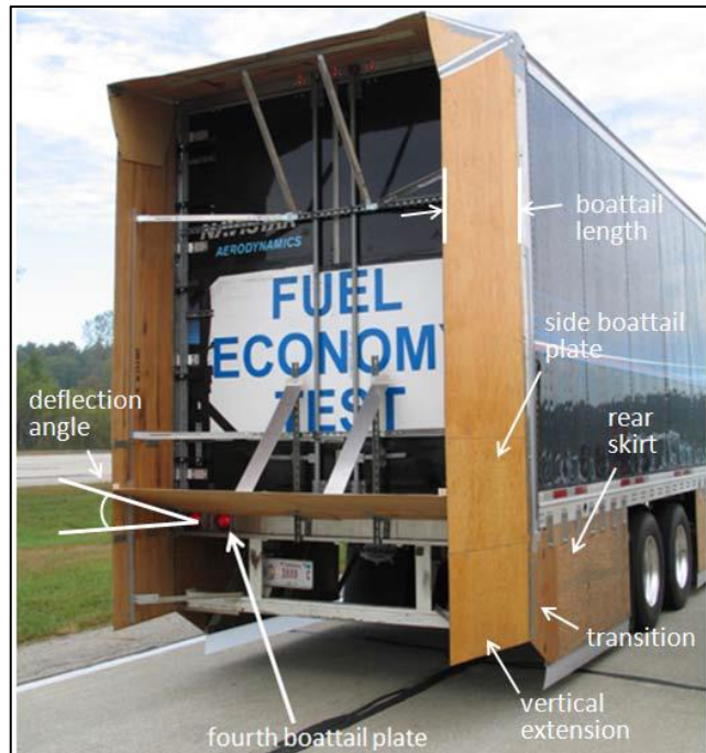
Figure 2.36: Six different combinations of devices on the semi-trailer truck model [53]
