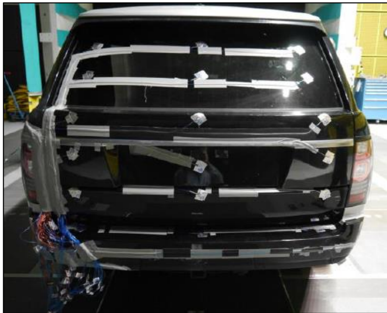
Figure 2.27: Surface pressure measurements on tailgate and rear screen [47]
