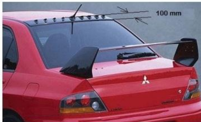
Figure 2.59: Position of vortex generators at the rear end of the roof [63]
