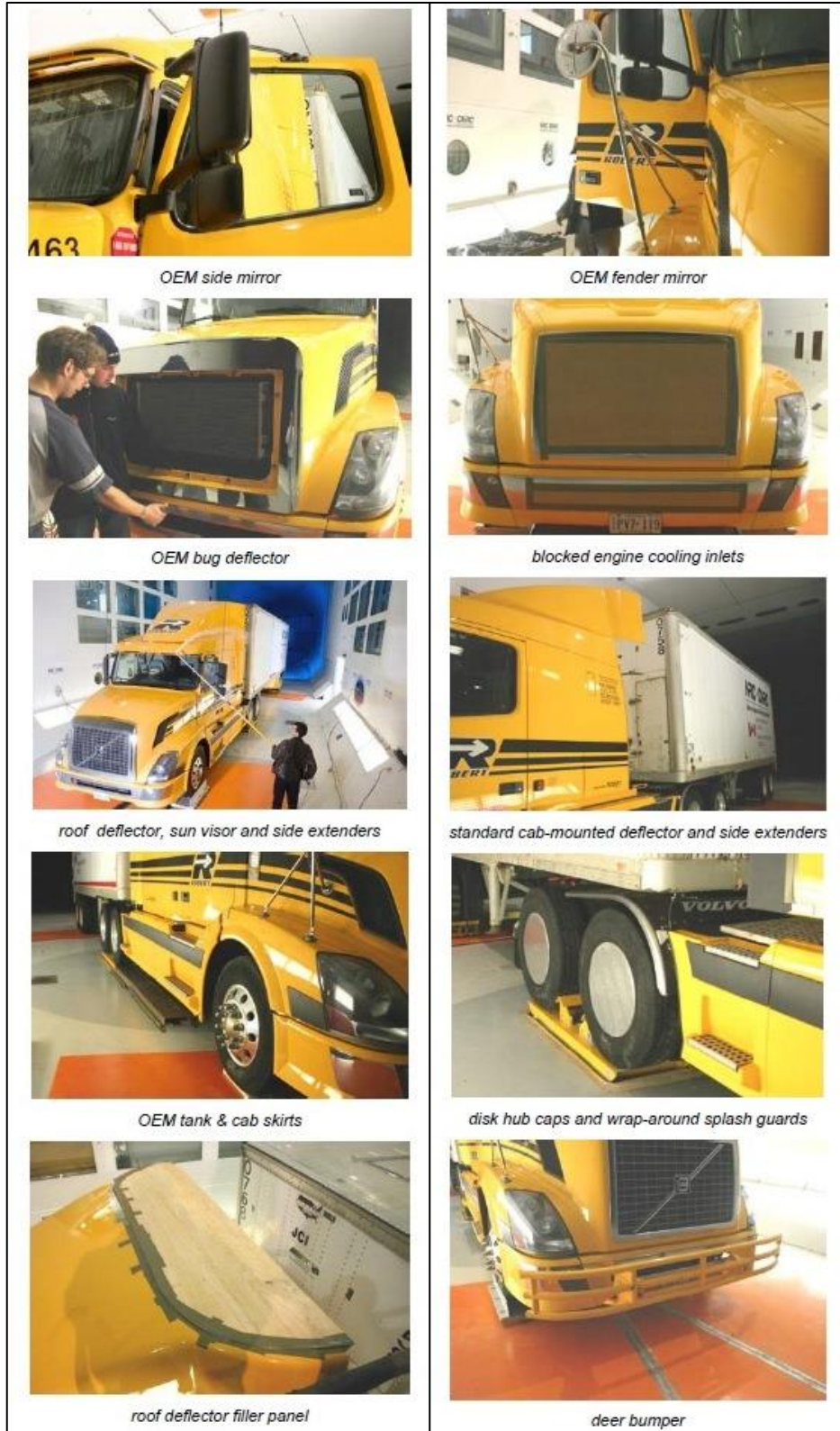
Figure 2.33: Common components of aerodynamic reduction techniques which were used in the tractor-trailer [51]
