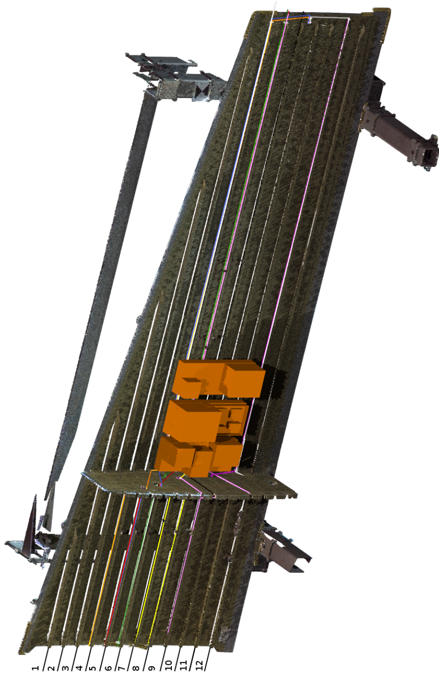
Figure 26: Render of completed wing skin assembly with numbered channels
