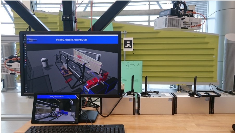
Figure 10.1: The Android and desktop client mounted within the real DAAC manufacturing cell
