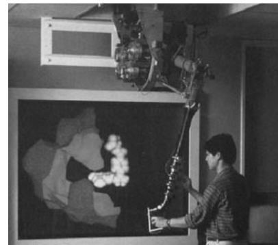
Figure 4.8: The GROPE I remote manipulator being used to test molecular interaction (BATTER et al., 1972)
