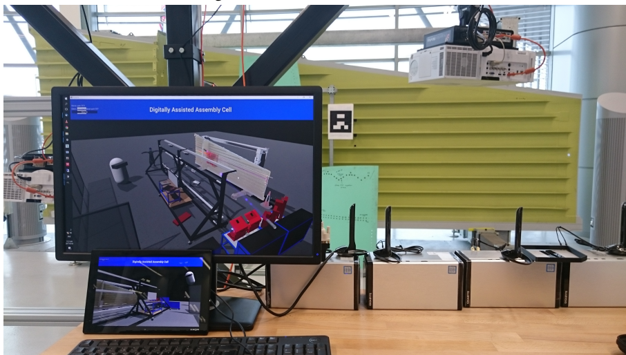
(c) The Android and desktop client mounted within the real world DAAC
