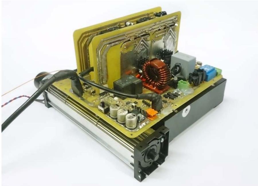
Figure 4.19. Prototype of proposed single-phase matrix converter
