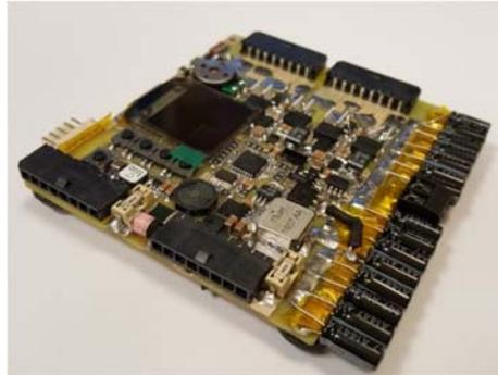
Figure 3.31. Assembled prototype converter showing its capacitor array.
