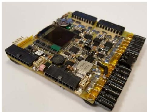
Figure 6.7: Prototype WPT transmitter employing phase shift based MEPT.
