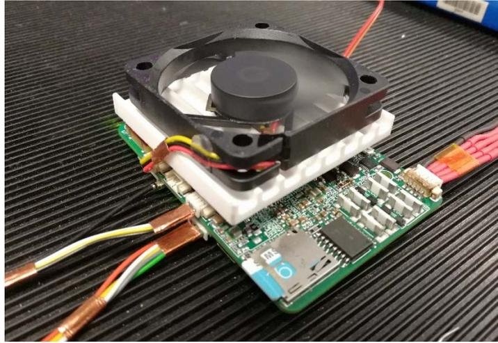
Figure 7.13. Wireless Power receiver showing connection to the prototype HyWi-FFTPLL shown in Figure 7.12 through the cable on the left.
