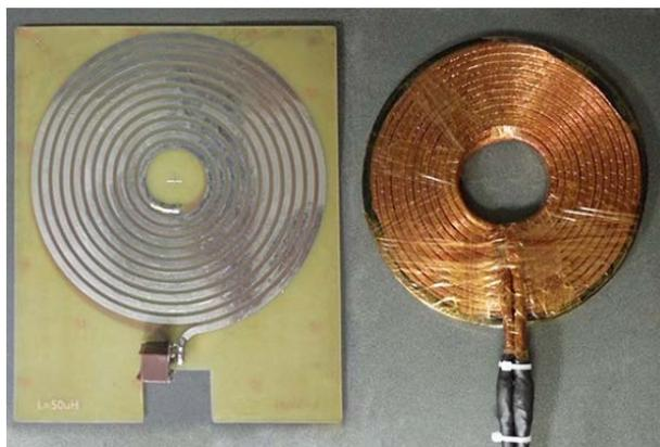
Figure 5.1. PCB coil and Litz wire coil for WPT system
