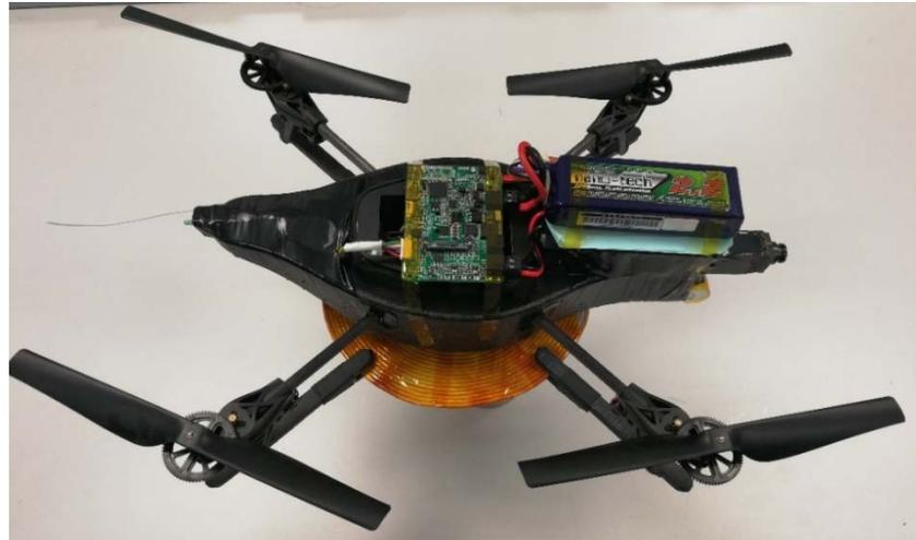
Figure 5.20. Evaluation of the WPT receiver on a drone platform, showing the example topology of the docking (wireless distance < 20cm) charging approach.
