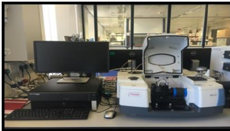
Figure 16: Photographic image of Thermo scientific™ Nicolet™ iS™50 FTIR spectrometer MTEC photoacoustic cell.
