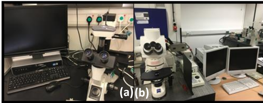
Figure 24: Photographic image of light optical microscopy (a) and confocal laser scanning microscope (CLSM) (b) respectively.
