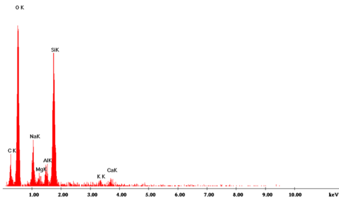
Figure 58: Micrograph of Leeds glass flakes Ltd UK based silicate glass sample composition energy dispersive x-ray spectroscopy (EDS) analysis.
