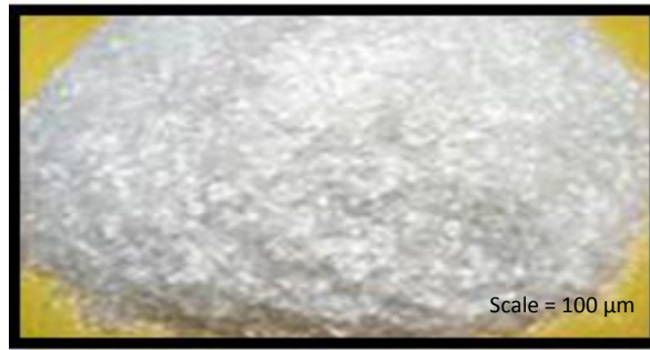
Figure 34: Photographic image of obtained silicate based glass flakes from Leeds Glass Flakes Company Ltd. UK.
