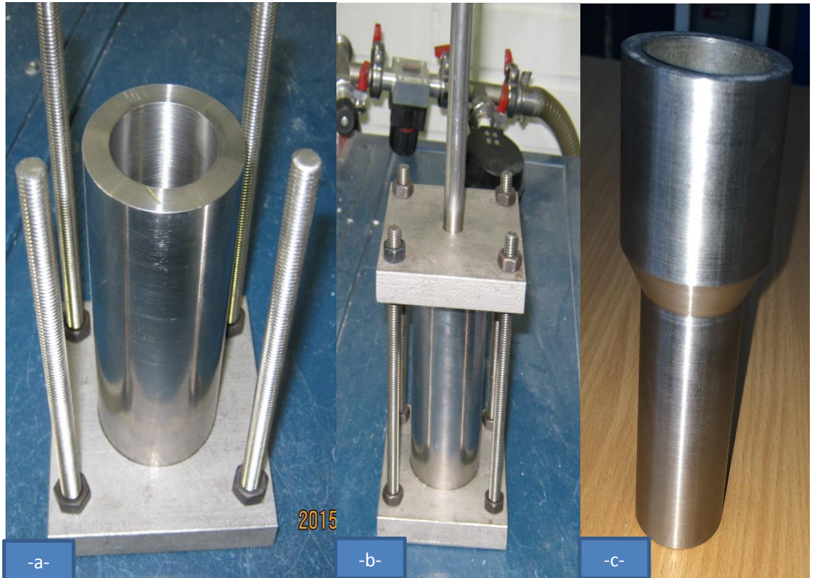
Figure (5-3): (-a-), (-b-) and (-c-) Steps of rig design for the infiltration system.
