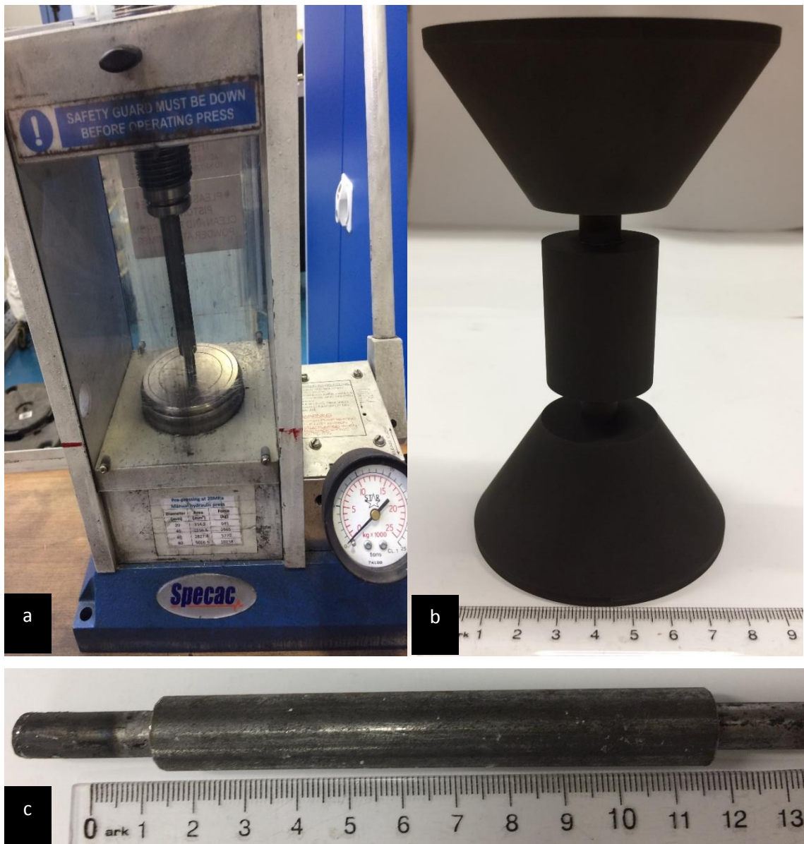
Figure (5-4): a) Press used to compact powder, b) SPS graphite mould and punches and c) PM mild steel mould and punches.
