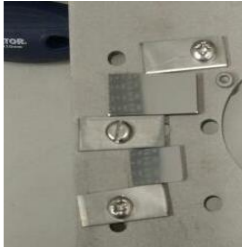
Figure 4-21 The position of the washers and substrates for "clean" coatings
