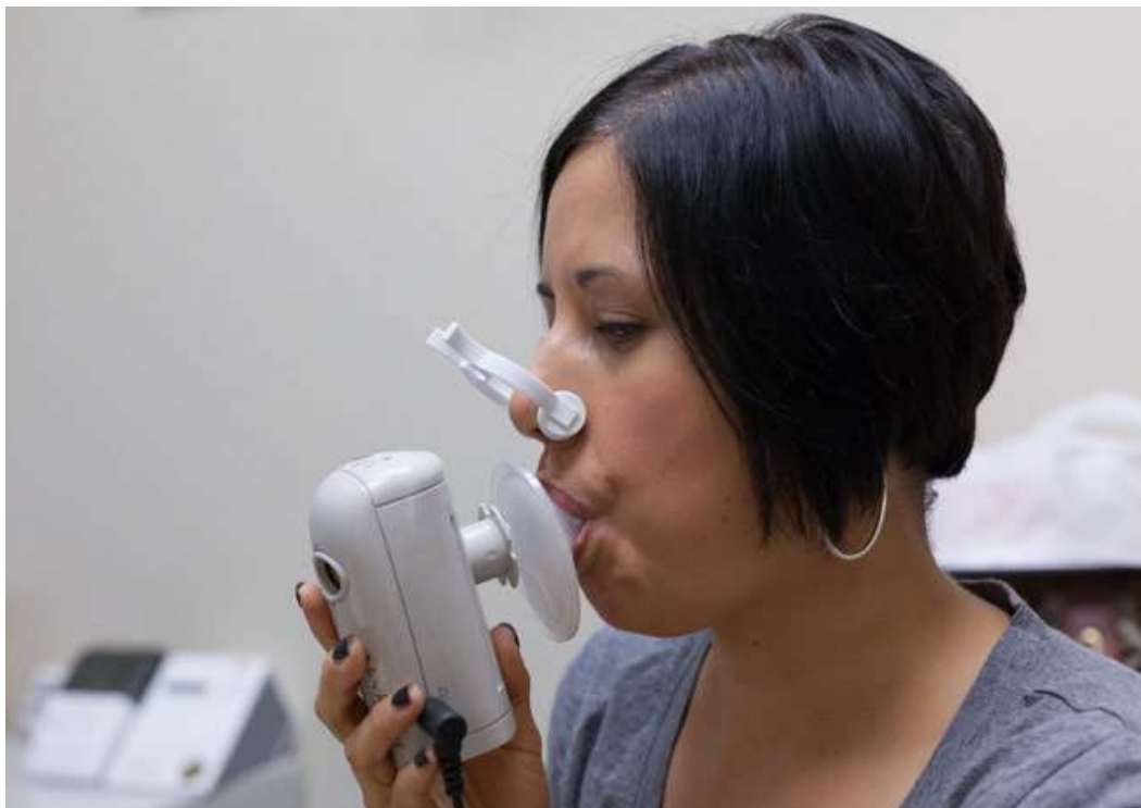
Figure 1.15. How to use a MedGem® handheld indirect calorimetry device to measure REE.
