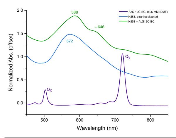
*Figure 3.22*: Extinction spectra for a plasmonic nanostructure array (NJ51) before and after adsorption of AcS-12C-BC. The extinction spectrum for AcS-12C-BC in solution is included for comparison.
