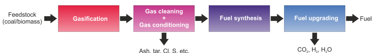
Figure 6. 1: General process flow for the industrial conversion of coal or biomass to SNG [183]. Adapted from Fuel, 89, J. Kopyscinski, T.J. Schildhauer, S.M.A. Biollaz, Production of synthetic natural gas (SNG) from coal and dry biomass - A technology review from 1950 to 2009, 1763-1783, Elsevier Ltd (2010), with permission from Elsevier.
