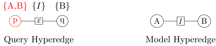
Figure 5.20: Example of one limitation of our simple relaxation system. Here the query graph (left) has two candidates (represented in curly brace) for its first node p . The elimination algorithm doesn't know that the other node q has only one candidate. The only thing known by the system is that one of the candidates ( I ) for the touching hyperedge x belongs to the set of neighbouring hyperedges of both A and B in the model. Therefore the system will not erase B from the candidate list of p .
