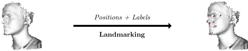
Figure 3.4: Problem: From a 3D mesh alone, detect the subset of vertices corresponding to 14 defined landmarks.
