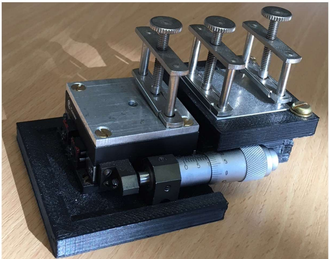
Figure 3.1 Home-built device for stretching and wrinkling PDMS
