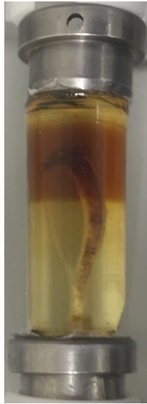
Figure 3.1. Mouse tibia embedded in acrylic resin.
