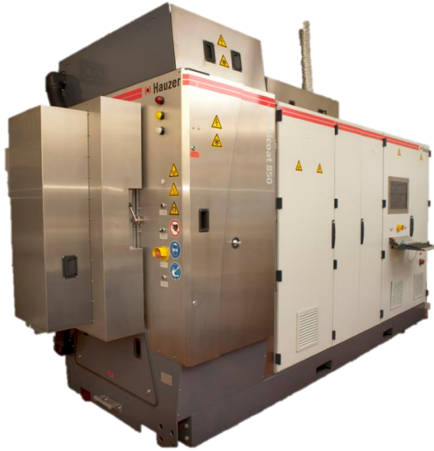
Figure 3.6 The Hauzer Flexicoat 850 deposition system
