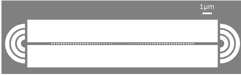
Figure 4.20: Digital image of a high-Q nanobeam PhCC with filling fraction, f , increasing linearly from the centre of the cavity over n_c = 15 , and with a further number, n_w = 15 , of holes with f held constant at the waveguide end, ready for fabrication.
