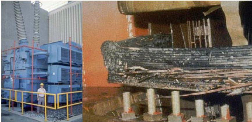
Figure 1.14: Transformer severe internal damage caused by the space storm of March 13 1989 in Quebec, Canada. The local population suffered an electrical power blackout in 1989. Credit: nasa.gov
