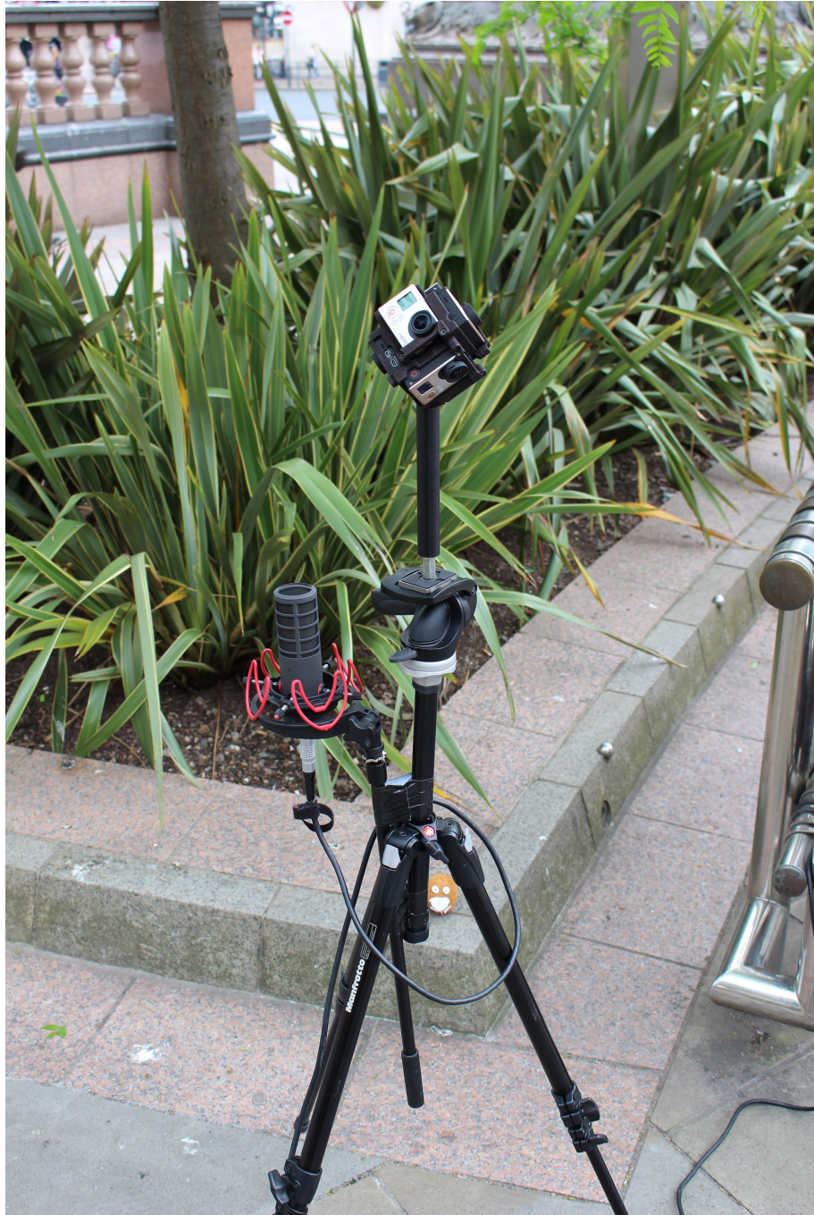
FIGURE A.11: The recording equipment in situ, including the Freedom360 GoPro rig and STM450 Soundfield microphone.
