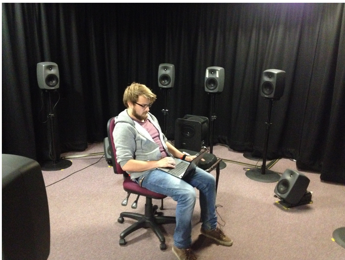
FIGURE 6.2: Test participant in the listening space. Note the surface provided for the test participant to rest their hand (with Shimmer device attached - see Section 6.1.2 for details) when the clips are played.
