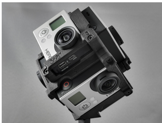
FIGURE 5.5: The ‘Freedom360 Mount’, an example GoPro mounting rig for the capture of 360° video. From [207].
