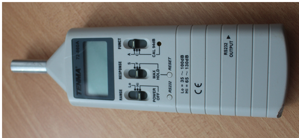
FIGURE A.13: The TENMA 72-860A sound level meter used in the recording work. The unit has a frequency range 31.5 Hz - 8 kHz [314].
