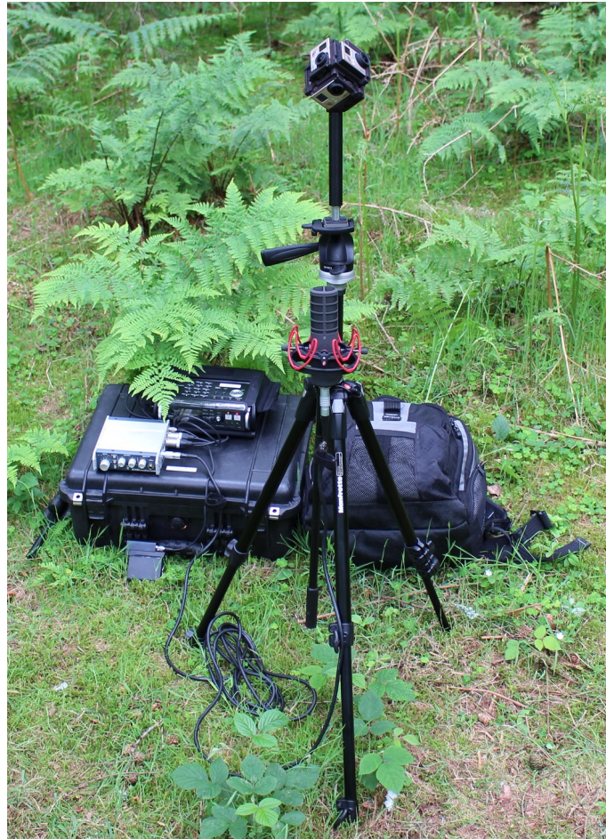
FIGURE A.12: Another view of the recording equipment, here indicating the portable recorder and Soundfield microphone pre-amp as well as the GoPro rig and the Soundfield microphone itself.
