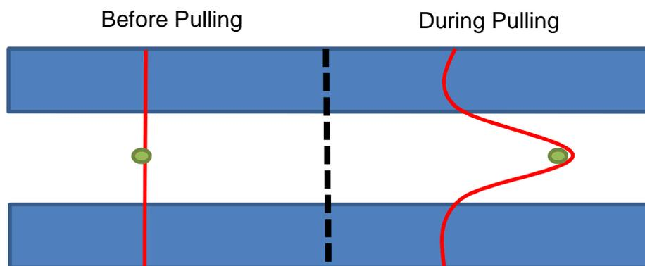
**Figure 7-1 Cartoon representation of lateral force AFM experiments.** Fibrin fibers (solid red line) are suspended between grooves (blue), the fiber can be pulled with an AFM cantilever tip (represented by a green circle). During pulling the fibers stretch and eventually rupture.
