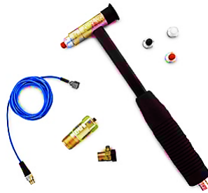
Figure 3.8: Impact Hammer, including different tips, cable and additional mass [1].
