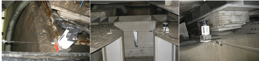
Figure 4.3: Extensimeters located at the north, center and south expansion joints in the bridge deck at the Saltash Tower [3].
